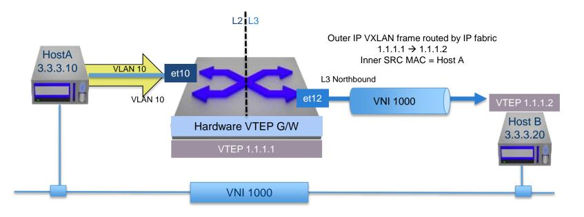
interface ethernet10 switchport switchport mode access switchport access vlan 10 ! interface ethernet11 switchport switchport mode trunk switchport trunk allow vlan 10,20 ! interface ethernet12
