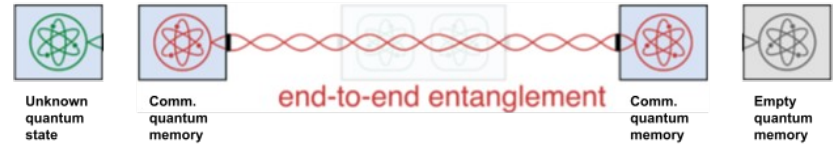
Step 2: Perform joint Bell state measurement (BSM) between unknown quantum state and end of the entanglement
